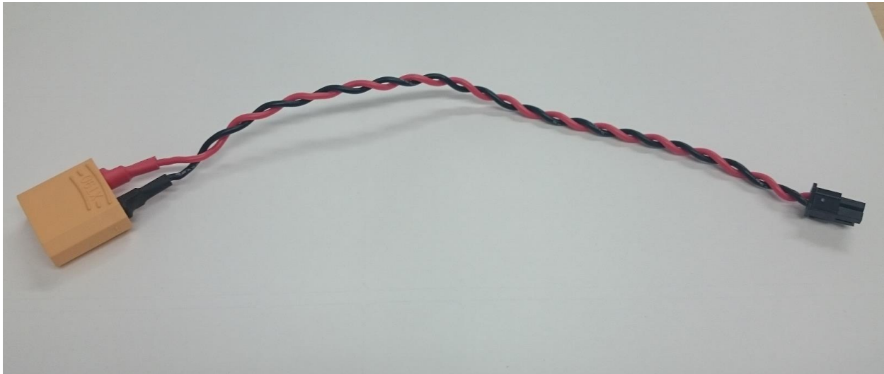
Figure 1. Incorrectly wired APS-WL-CAB-POWER-XT90-R1. Destroy or dispose of as soon as possible.
