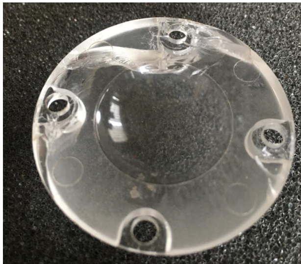
Figure 1. Large crack close to screw mounting holes
