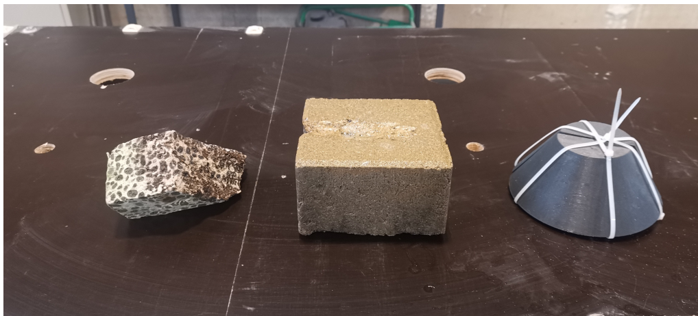
Figure 4.3: Targets used for the B-scans sections. On the left, an irregularly-shaped rock approximately 3.5 centimeters high and 7 centimeters long, in the middle, a 4*10*12 cm concrete brick, and on the right, a 3D-printed Manta mine with 4 centimeters high, with a large diameter of 10 centimeters and a small diameter of 4 centimeters.
