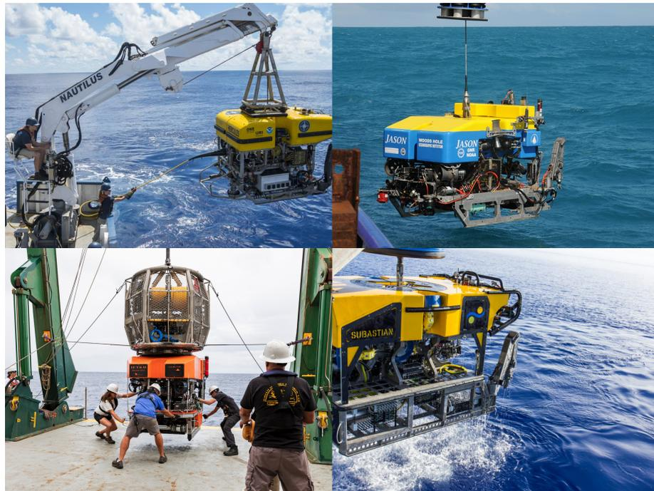
Figure 1.2: Clockwise from top left: Hercules [7], Jason [8], SuBastian [9], and Lu'ukai [10] are examples of research remotely operated vehicles (ROVs) currently in service.
