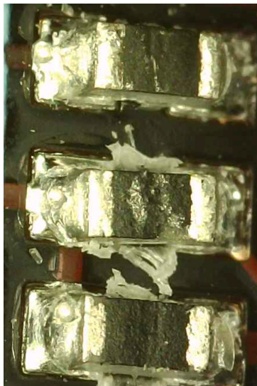
Figure 3: Damaged 0402 size 100k resistors reading open circuit
