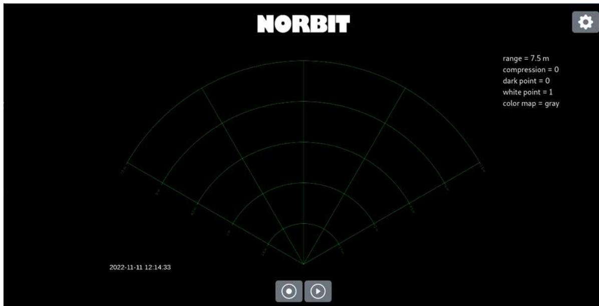
When play button is pressed, the sonar starts pinging and the button changes to a stop button
