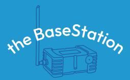
The BaseStation is a wifi radio access point for the BlueBoat with a 2.4 Ghz MikroTik radio, internal battery and charge management, and USB-C connectivity.
