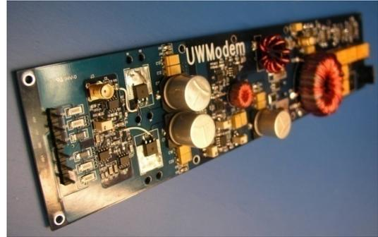
Figure 8. Analog Transceiver
