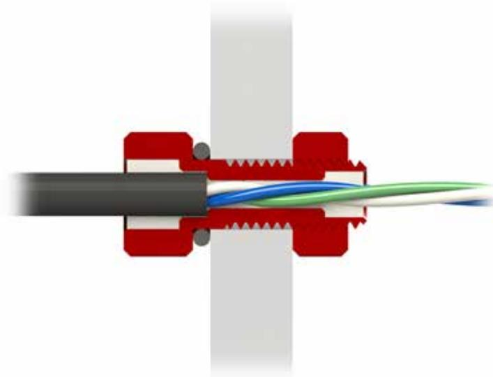
Figure 2 - Cut-away of penetrator and cable
