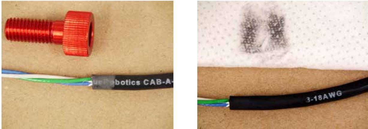
Figure 4 - Sanded and Cleaned Cable
