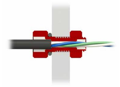
Figure 2 - Cut-away of penetrator and cable
