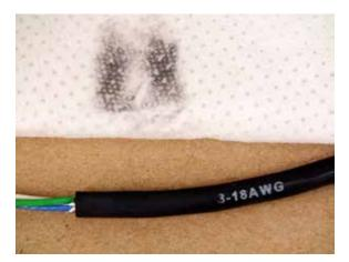
Figure 4 - Sanded and Cleaned Cable
