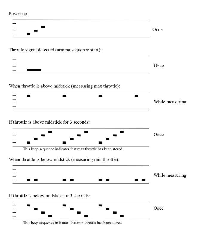
At this point throttle calibration values are stored. You may remove power from the ESC, or just continue running your ESC.
