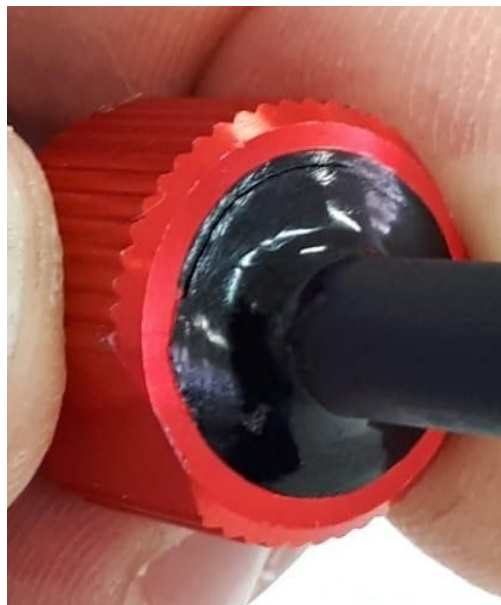
Figure 3. Cable Penetrator with poor adhesion to aluminum cable penetrator.
