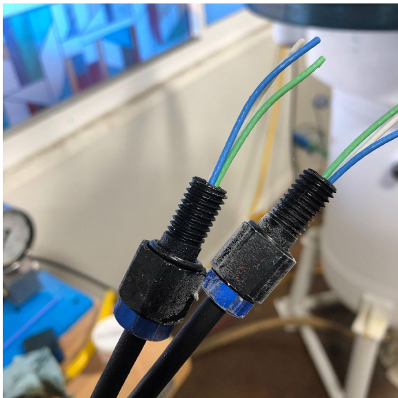
Compression gland penetrator prototypes after <0^{\circ}\text{C} exposure (left) and our pressure test chamber cooled to <5^{\circ}\text{C} for cold water testing (right).
