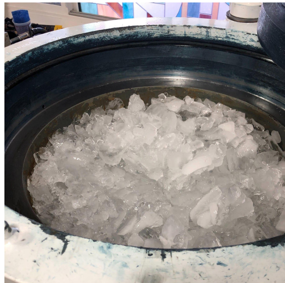
Compression gland penetrator prototypes after <0^{\circ}\text{C} exposure (left) and our pressure test chamber cooled to <5^{\circ}\text{C} for cold water testing (right).
