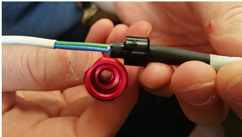
Figure 1. Cable Penetrator with poor adhesion to aluminum cable penetrator.
