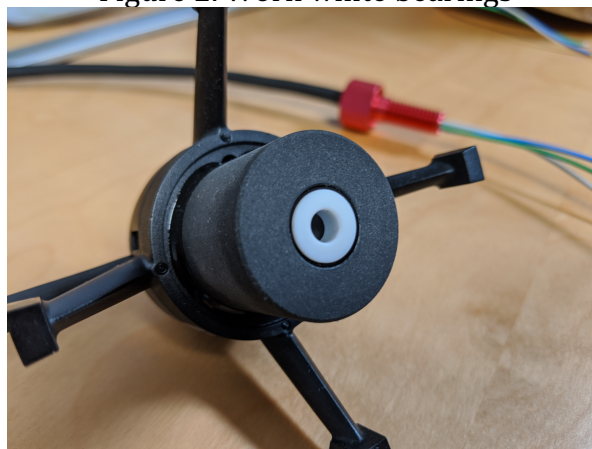
Figure 3. White bearing on a potted thruster stator.
