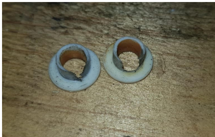
Figure 2. Worn white bearings
