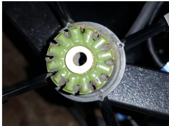
Figure 1. Worn white bearings on a T200 with a green epoxy stator.
